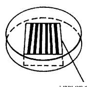
i INE OF CONTACT Straight bands equally spaced and parallel, indicate that the surface is flat within 11.6 millionths of an inch.
